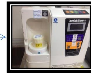
5) Place the CPU in the machine where the filter was.
