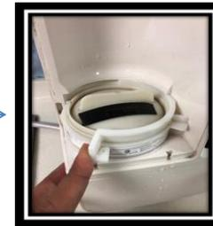
5) Place the **Cleaning Cap** in the machine where the filter was.
