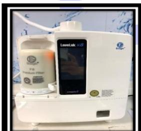
20) Put your filter back in (When storing your Cleaning Cap don't store it wet with the lid on, allow it to completely dry.)
