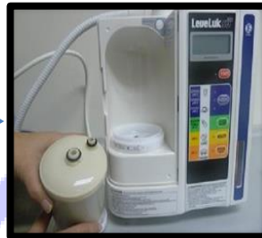
3) Remove the filter
