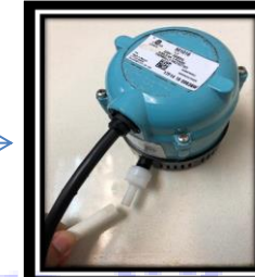
17) Disconnect white hose from pump hose.
