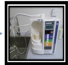
18) Connect white hose to tap water. Then rinse the machine by running water for 5 minutes
