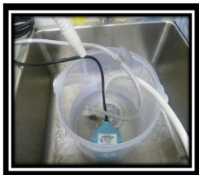
13) Place pump and acidic hose (grey hose) into the container.
