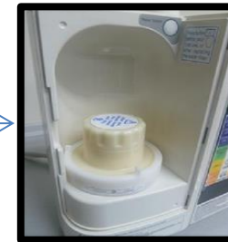
5) Place the CPU in the machine where the filter was.
