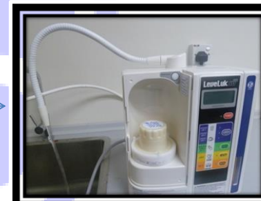
9) Rinse the machine by running water for 5 minutes with the CPU still in place.
