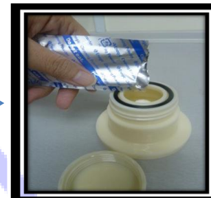
4) Take out CPU-N and fill in 1 sachet cleaning powder
